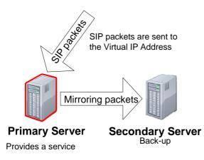
2. If the Primary server goes down, the Heartbeat feature switches the Seconday server to be the Primary server and assigns the Virtual IP address to the new Primary server.
