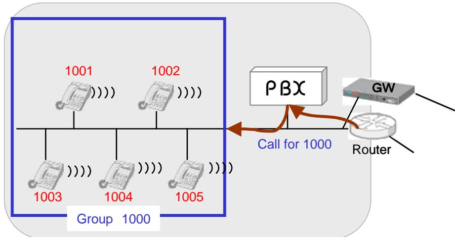
In this example, a Ring Group is set up for extension 1000. When calls are received by any extension in the group, all extensions (1001-1005) ring simultaneously.
