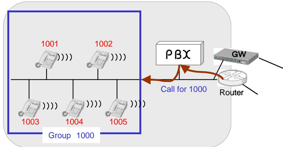
In this example, Ring Group is set up for extension 1000. When calls are received by any extension in the group, all extensions (1001-1005) will ring simultaneously.
